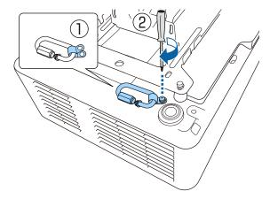
Loop the safety wire through the hole in the ceiling mount, and then attach both ends to the carabiner.
