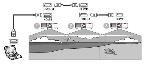
Connect the projector to the computer using the HDMI cable, and then connect the HDMI1 port and HDMI Out port of the projectors using the HDMI cable.
