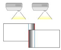
• Select the **Blend Curve** setting and select a gradient for the shaded area on the projectors.
